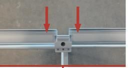
**6.** Place the frame on the ground and slide in the aluminium bars from the side.
